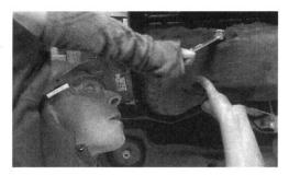
6. While the oil drains you can begin removing the oil filter.
